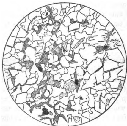
FIGURE 8.—Thin section of hematite quartzose dolomite from Swanton. Dotted particles are quartz; black are magnetite; shaded areas are hematite stain; a black-banded particle is plagioclase, a long-streaked one, muscovite; the rest are dolomite. Enlarged 77 diameters.
