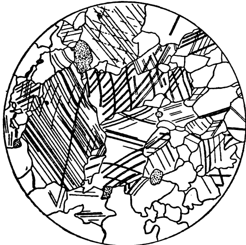
FIGURE 1.—Thin section of white calcite marble from the Goodale or Girard College quarry in Sheffield, Mass., with flexed twinning planes due to secondary compression. Texture very coarse and irregular. Dotted particles are quartz. Enlarged 20 diameters. This quarry supplied columns for Girard College, in Philadelphia. The curvature of the calcite plates can be detected, even in a hand specimen.
