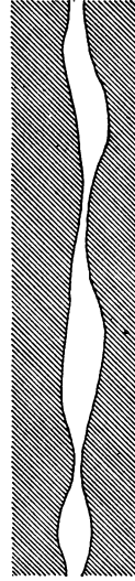
POCKET AND PINCHES RESULTING FROM SLIP- PING OF UNEVEN WALLS OF FISSURE.
