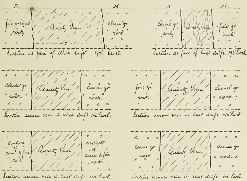
Fig. 10. Cross sections on the Reimer vein in Shaft No. 1, showing character of the wall rocks.
