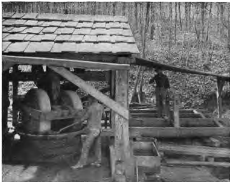
CHILIAN DRAG-MILL AND ROCKERS, NEAR GOLD HILL, N. C.
