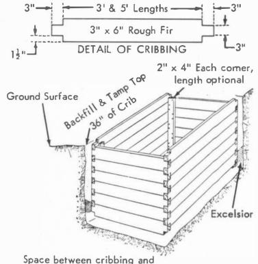
Space between cribbing and test pit walls to be backfilled with excelsior when exploring loose ground.
