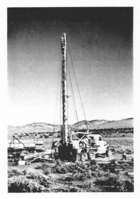
FIGURE 8. - Truck-mounted Keystone Model 70 placer drill.
