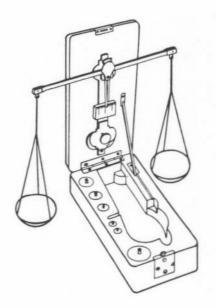
FIGURE 20 – A folding assay balance widely used in placer work. Capacity 10 grams, sensitive to ¼ milligram. Complete in mahogany case with set of weights 10 grams by 1 milligram. Size when closed, about  $6x3x1\frac{1}{2}$  inches.
