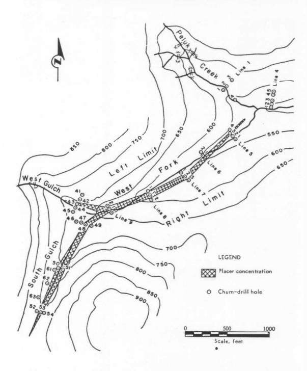
FIGURE 11. – Typical drilling pattern for prospecting narrow, stream-type deposits. (From USBM R.I. 6587).
