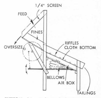
FIGURE 19 – Schematic diagram showing the arrangement of a typical hand-operated dry washer. In use, the dirt is moved over the riffles by puffs of air forced through the cloth bottom by the bellows. The gold lags behind and accumulates along the upstream edges of the rif fles.
