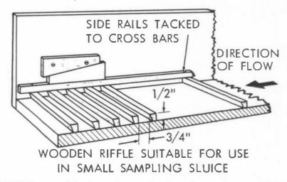
FIGURE 17. - Wooden riffle suitable for use in a sampling sluice.
